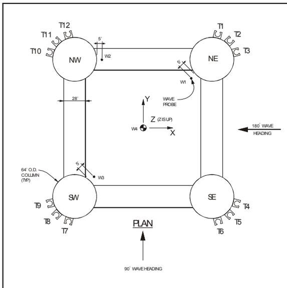
Figure 2 Wave Heading and Coordinate Definition
