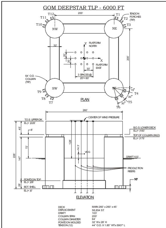
Figure 1 TLP Hull Configuration
